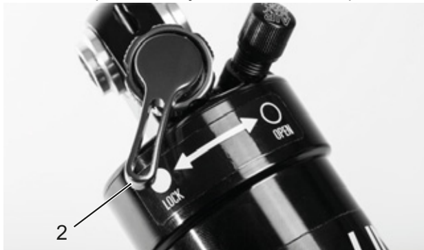
Figure 80: Suntour compression adjuster closed (2)
