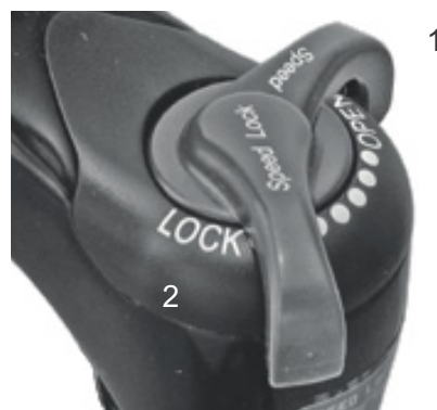
Figure 78: Suntour compression adjuster with the OPEN (1) and LOCK (2) positions
