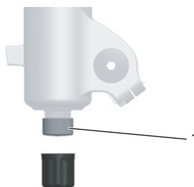
Figure 61: FOX rebound adjuster (1) on the fork
