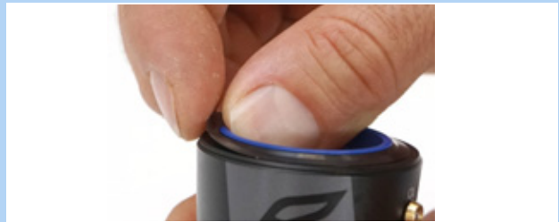
Figure 193: Detaching the seal lip ring
