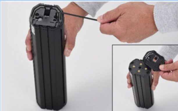
Figure 53: Detaching the upper interface
