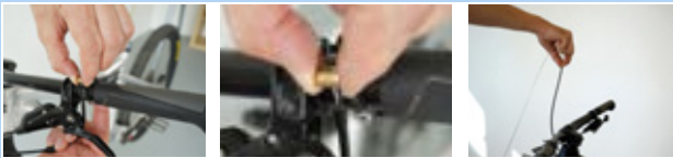
Figure 189: Unfastening the remote control
