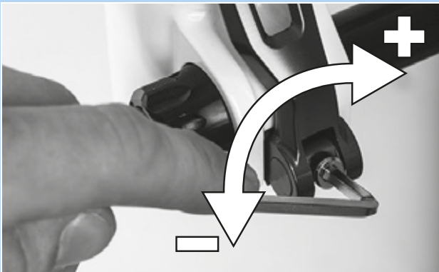
Figure 148: Adjusting the quick release clamping force
