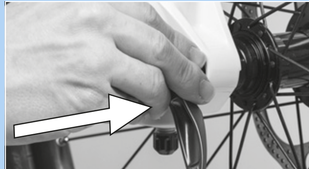
Figure 73: Inserting the quick release in the direction of the arrow
