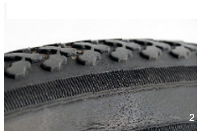
Figure 138: Examples of fatigue cracks (1) and ageing cracks (2)
