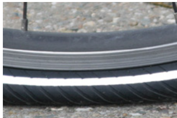
Figure 98: Much too little tyre pressure
