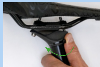
Figure 206: Closing the height adjustment
