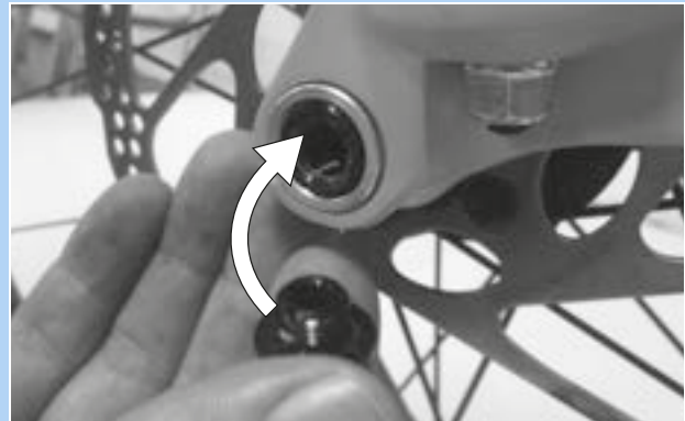
Figure 64: Pushing the quick release lever into the axle
