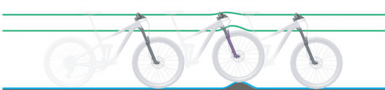
Figure 126: Optimum performance over bumps
