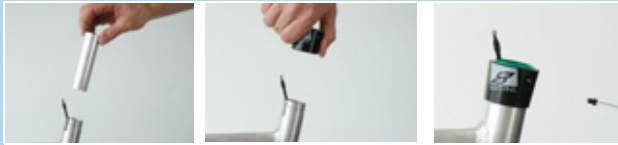
Figure 174: Fitting the slide bushing and outer sleeve
