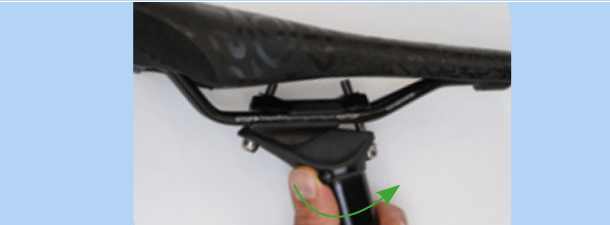
Figure 201: Opening the height adjustment
