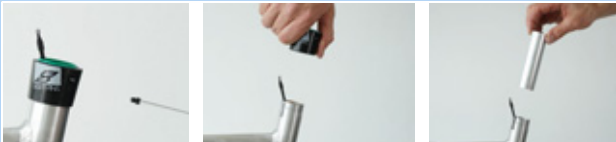
Figure 158: Removing the outer sleeve and slide bushing
