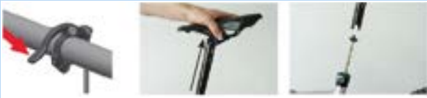
Figure 151: Pulling the seat post out
