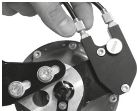
Figure 143: The tension adjuster on Rohloff hub versions with external switch control is located on the cable box positioned on the left-hand side
